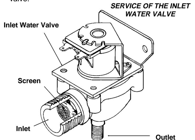
Check the screen of the valve, it may be clogged and is restricting the flow of water into the machine. If that is the problem, clean the screen and reverse the steps so far to reassemble.
