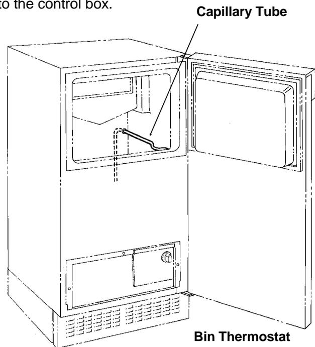
8. Remove the wires attached to the bin thermostat.
