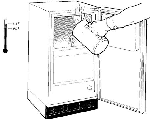
7. Clean the bin liner of mineral scale by mixing some ice machine cleaner and hot water, and using that solution to scrub the scale off of the liner.
