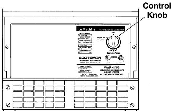
5. Allow the unit to operate for 1 hour, and check the size of the cubes, if they are not correct, adjust as recommended on page 17.
