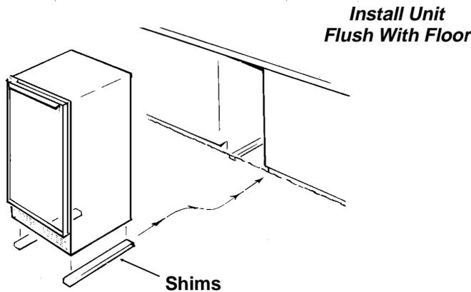
If a floor is to be installed after the ice machine, shims the thickness of the floor should be installed under the DC33 to keep the machine level with the floor. Also, allow 1/8" clearance on each side of the cabinet.
